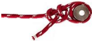
Figure 11: Round turn & 2 1/2 hitches
