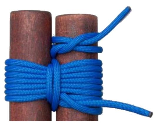
Start with a Clove Hitch around one pole. Twist short end around long and wrap the rope around both poles, alternately going over and under each pole about three or four turns. Tighten the lashing by surrounding it with three or four frapping turns. Finish with a final Clove Hitch.
