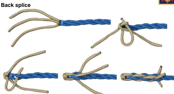
A back splice is used where the strands of the end of the rope are spliced directly back into the end without forming a loop. It is used to finish off the end of the rope to keep it from fraying. The end of the rope with the splice is about twice the thickness of the rest of the rope. With nylon and other plastic materials, the back splice is often no longer used; the rope strands are simply fused together with heat to prevent fraying.
