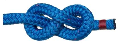
The figure of eight knot is used as a stopper knot at the end of a rope to prevent the end passing through an eye or a pulley.
